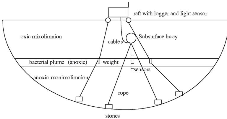
Fig. 2. Installation of the sensors in Lake Cadagno (for details see 'Materials and methods')
