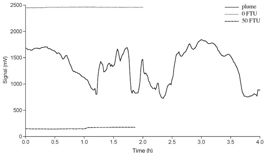
Fig. 3. Calibration of optical sensors. Time course of signal of a turbidity sensor *in situ* (bacterial plume in Lake Cadagno) and in calibration liquids of 0 and 50 FTU (formazine turbidity units) in the laboratory. Signal output was also calibrated in FTU units
