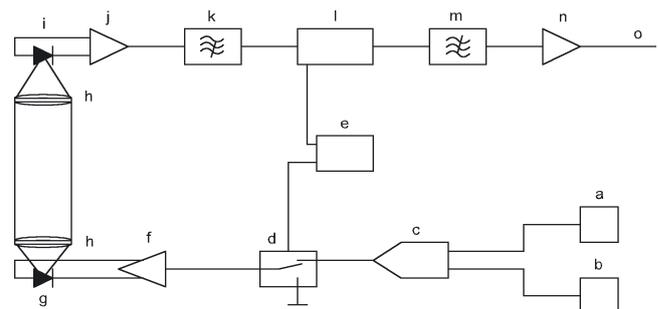
Fig. 1. Schematic overview of the electronic circuit of the turbidity-temperature sensor. a: voltage reference; b: temperature sensor; c: adjustable adding amplifier; d: modulator switch; e: oscillator; f: voltage to current converter; g: LED (light-emitting diode); h: lens; i: pin photodiode; j: pre-amplifier; k: highpass-filter; l: synchronous demodulator; m: low-pass filter; n: output amplifier; o: output voltage, 0 to 3 V
