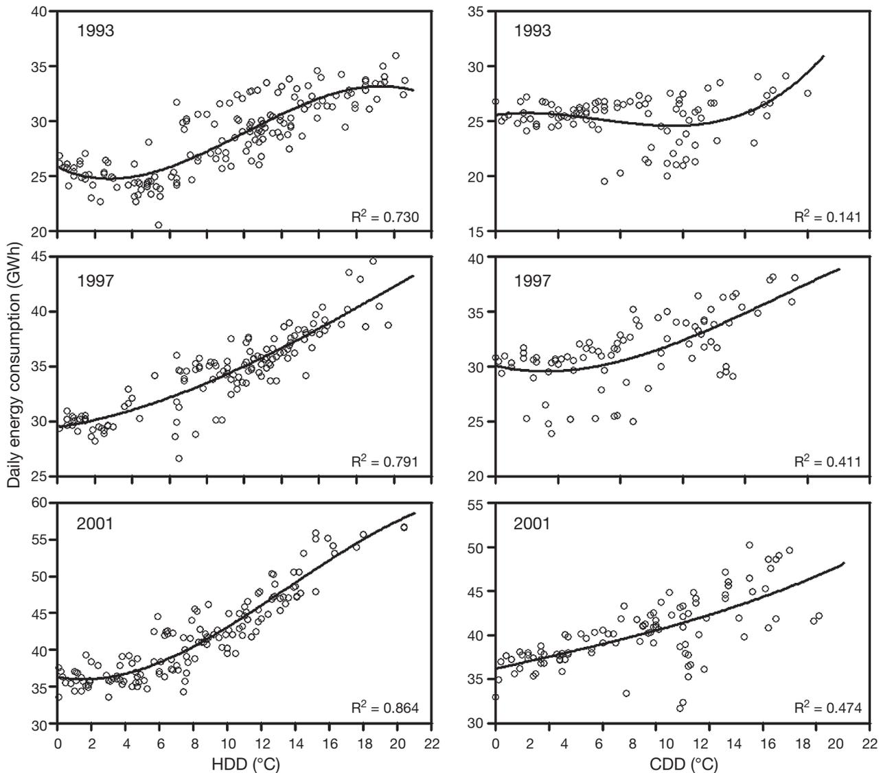
Fig. 10. Daily energy consumption with HDD and CDD for working days only and for years 1993, 1997 and 2001. Black lines: best fit curves;  $R^2$ : correlation coefficients
