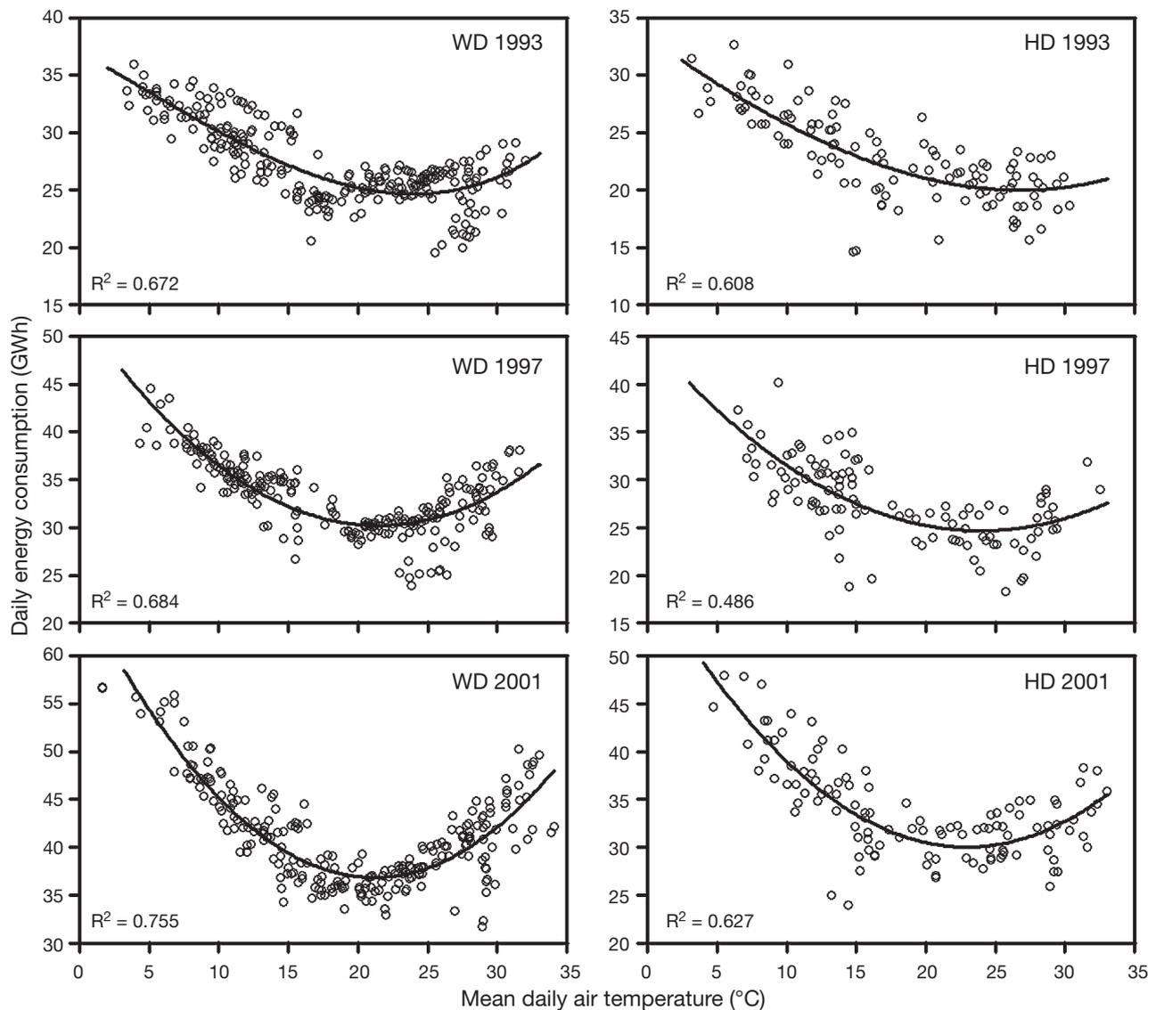
Fig. 8. Correlation plots of daily energy consumption and mean air temperature for 1993, 1997 and 2001 on working days (WD) and weekends/holidays (HD). Black lines: best fit curves;  $R^2$ : correlation coefficients
