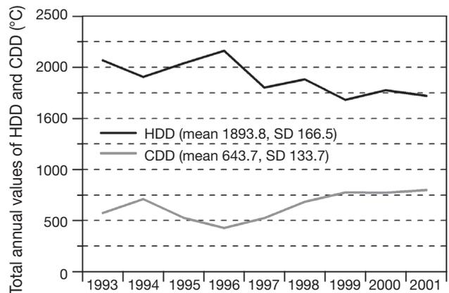
Fig. 9. Total annual variation in heating degree-days (HDD) and cooling degree-days (CDD) for 1993–2001 using 22°C as base temperature
