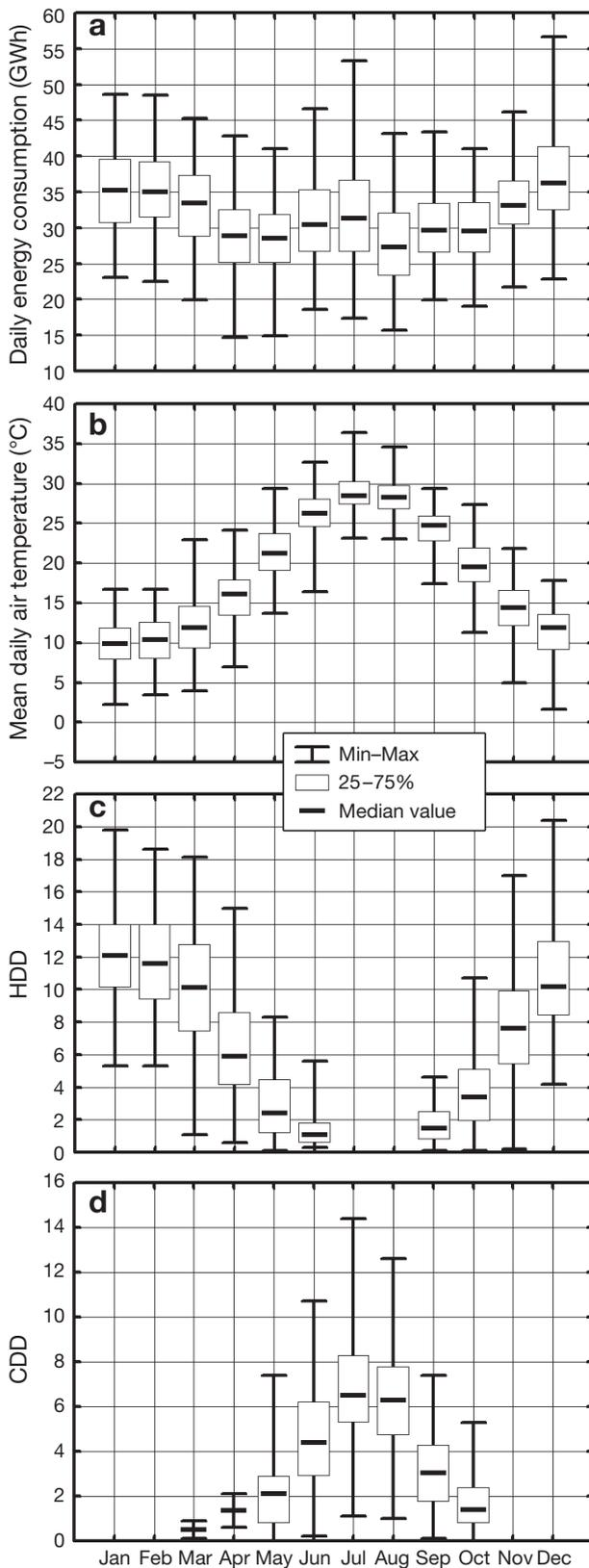
Fig. 11. Box-whisker plots for (a) daily energy consumption, (b) daily mean air temperature, (c) HDD and (d) CDD, 1993–2001
