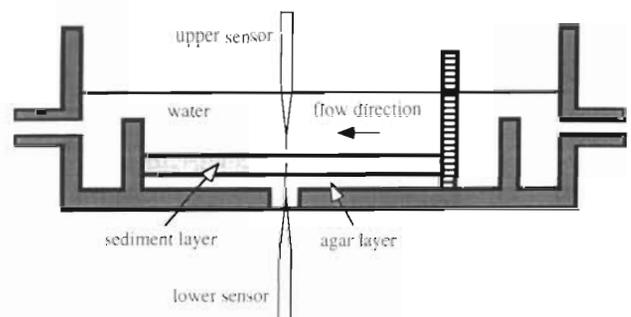
Fig. 1. Rectangular flow chamber used in the experiment. The agar-filled hole in the bottom of the chamber made it possible to measure with 2 microelectrodes along the same vertical axis
