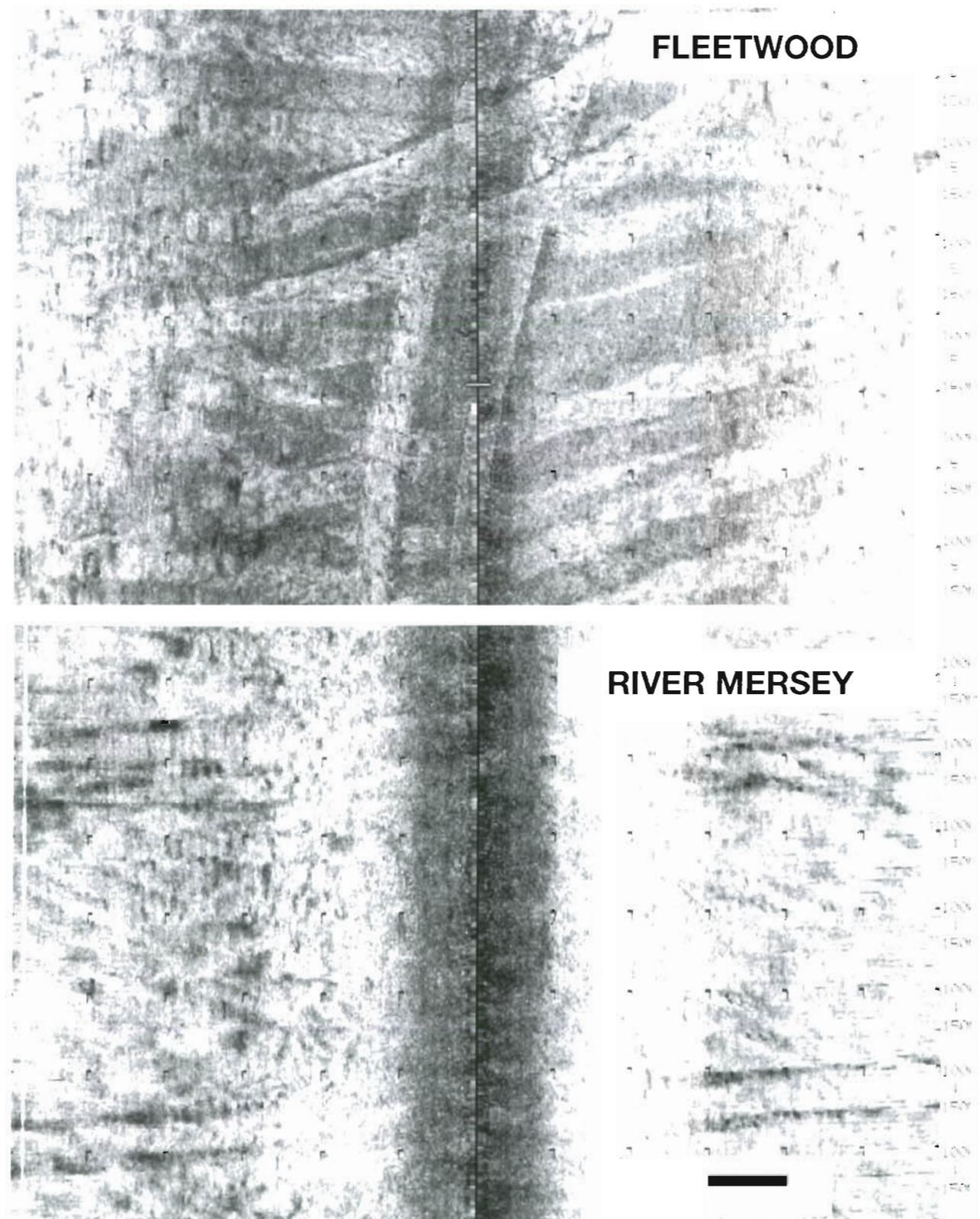
Fig. 3. A portion of the side-scan sonar record showing pairs of 12 m wide beam trawl marks on muddy ground off Fleetwood, and pairs of 4 m wide beam trawl marks off the River Mersey. The trawl marks run in a north/south direction. Scale bar = 25 m
