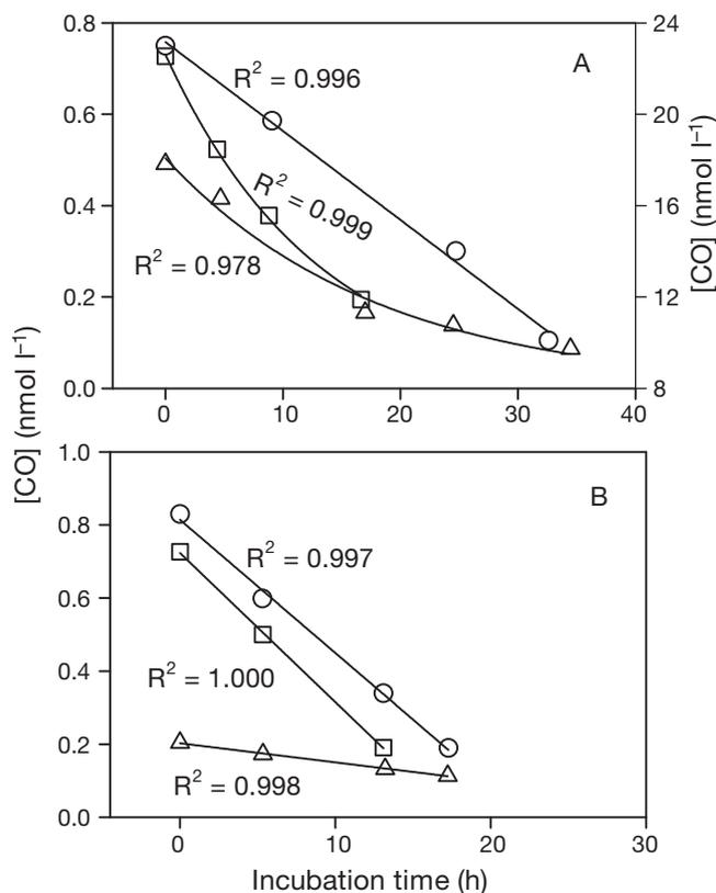
Fig. 3.  $[\text{CO}]$  versus incubation time plots showing saturation (straight lines) and first-order (curved lines) kinetics of  $\text{CO}$  uptake at (A) Stn SF (Saguenay Fjord) and (B) Stn 12 for 3 depths: 2 m (O), 10 m (□) and 20 m (Δ).  $[\text{CO}]$  at 2 m in (A) is on the right y-axis scale. Lines are the best fit plots of the data
