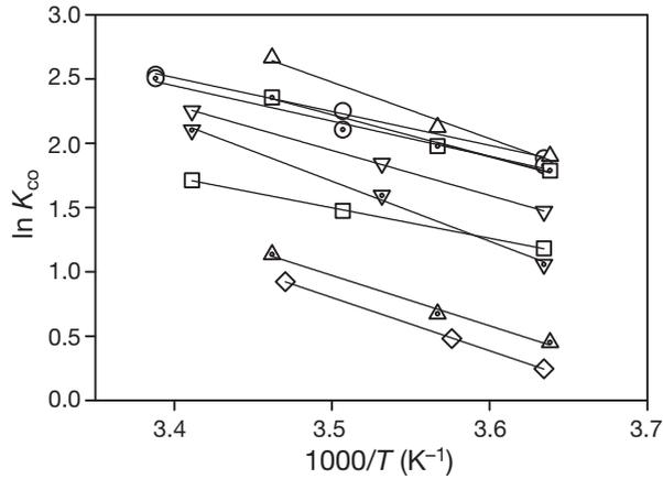
Fig. 4. Arrhenius plots of first-order CO uptake rate constant ( $K_{\text{co}}$ ) for Stns 1 (O), 2 (◊), 3 (□), 7(◻), 9 (Δ), 11 (▲), SF at 2 m (▽), SF at 9 m (∇) and SU1 (◇). Lines are the best fit plots of the data. Coefficients of determination ( $R^2$ ) and activation energies derived from these plots are shown in Table 2.  $T$ : temperature; see Table 1 for station abbreviations
