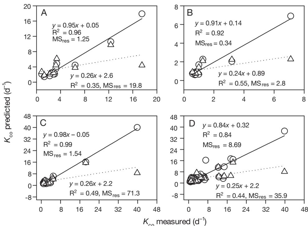
Fig. 7. First-order CO uptake rate constants ( $K_{co}$ ) predicted from the equation  $\ln K_{co} = \ln[BC] + A \times T^{-1}$  versus measured  $K_{co}$  values after (O and solid lines) and before ( $\Delta$  and dotted lines) taking into the particle effect for (A) autumn, (B) winter, (C) spring, and (D) all 4 seasons combined. Data are from all stations, including Stn 2 in the turbidity maximum zone. Lines are the best fits of the data.  $MS_{res}$  is the residual mean square
