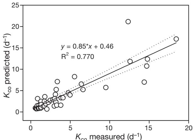
Fig. 6. First-order CO uptake rate constants ( $K_{co}$ ) predicted from the equation:  $\ln K_{co} = \ln[BC] + A \times T^{-1} + Y_0$  (Table 3) versus measured  $K_{co}$  values for all-season data. Solid line is the best fit plot of the data and broken lines are 95% confidence intervals. Data from Stn 2 in the turbidity maximum zone are excluded for autumn, winter and spring
