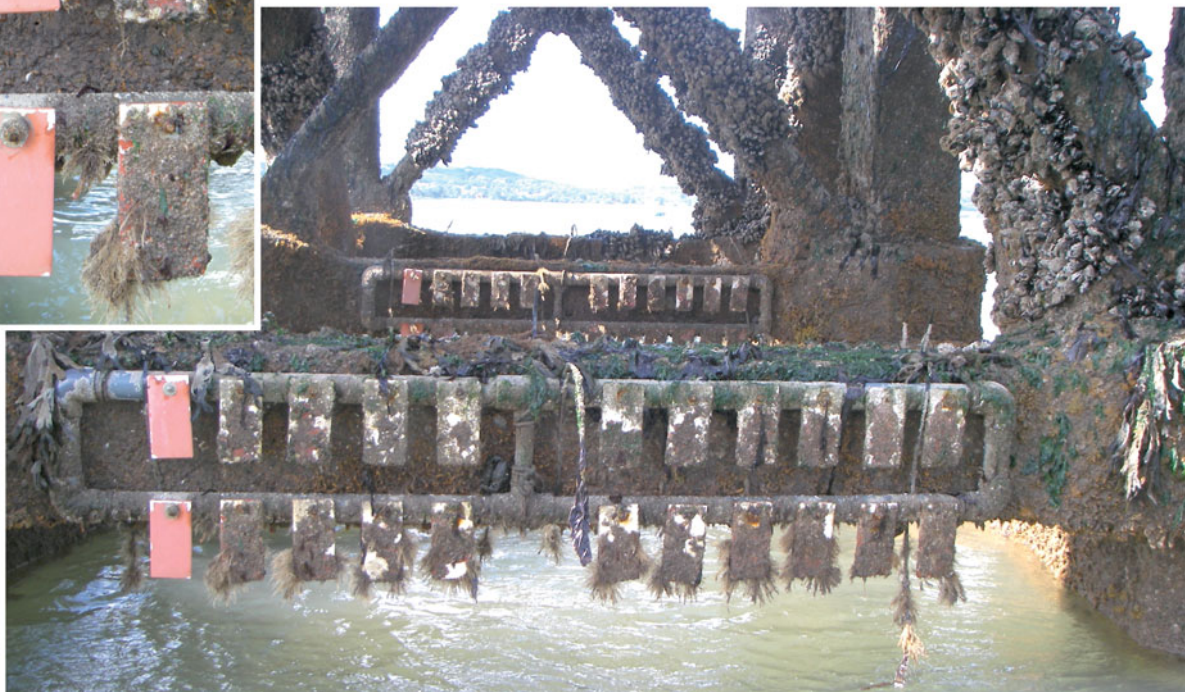
Fig. 5. In situ settlement frames at Mumbles Pier after 18 wk immersion. Second frame is shown in the background. A third settlement frame is secured to the farthest strut, facing the other direction. Treatments were replicated 3 \times at each location on 2 substrates: steel panels and ceramic tiles. The lead frame shows 2 replicate rows of tiles with experimental numbers (see Table 1) from left to right. The positive controls are barren while all other tiles are heavily fouled by the barnacle Semibalanus balanoides and algae. Inset shows greater detail of the positive (left) and negative (right) controls
