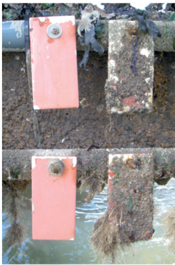
Fig. 5. In situ settlement frames at Mumbles Pier after 18 wk immersion. Second frame is shown in the background. A third settlement frame is secured to the farthest strut, facing the other direction. Treatments were replicated 3 \times at each location on 2 substrates: steel panels and ceramic tiles. The lead frame shows 2 replicate rows of tiles with experimental numbers (see Table 1) from left to right. The positive controls are barren while all other tiles are heavily fouled by the barnacle Semibalanus balanoides and algae. Inset shows greater detail of the positive (left) and negative (right) controls
