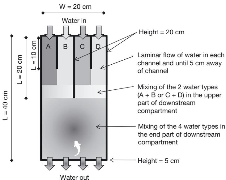
Fig. 1. Four-channel choice flume. Four tanks were simultaneously connected to the 4 upstream channels (A, B, C, and D) by pipes to create constant gravity-driven flow into each channel. See 'Materials and methods' for further details
