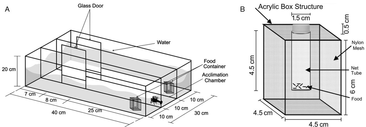
Fig. 1. Aquarium and container design for tests of food attraction with the redclaw crayfish *Cherax quadricarinatus*. (A) glass aquarium device showing the position of the glass doors, acclimation chamber, water level and food container positions; (B) food container device
