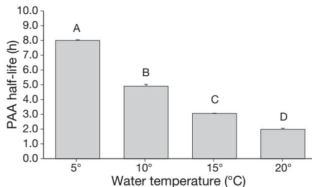
Fig. 2. Calculated PAA half-lives (mean  $\pm$  SD) in full-strength seawater at 4 different temperatures, based on data from PAA decay with a nominal concentration of  $1 \text{ mg l}^{-1}$  PAA. Different letters denote significant difference ( $p < 0.01$ )
