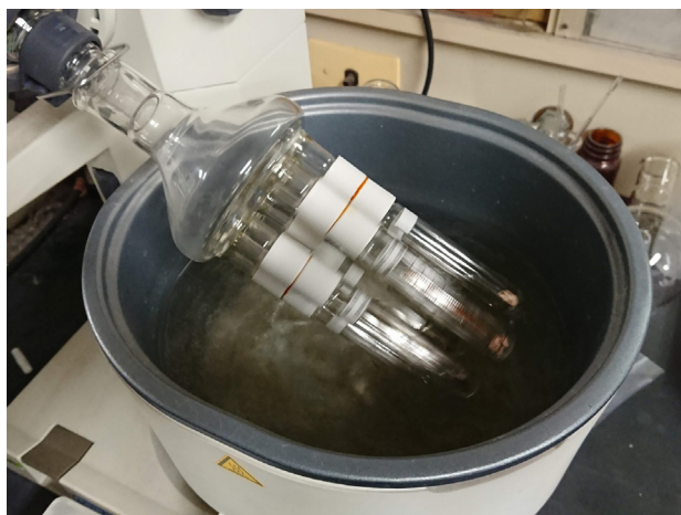
Fig. 1. Rotary evaporator equipped with a custom adaptor for drying 6 samples simultaneously
