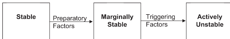
Fig. 1. Concept of progressing conditions influencing landslide initiation (Crozier 1989)
