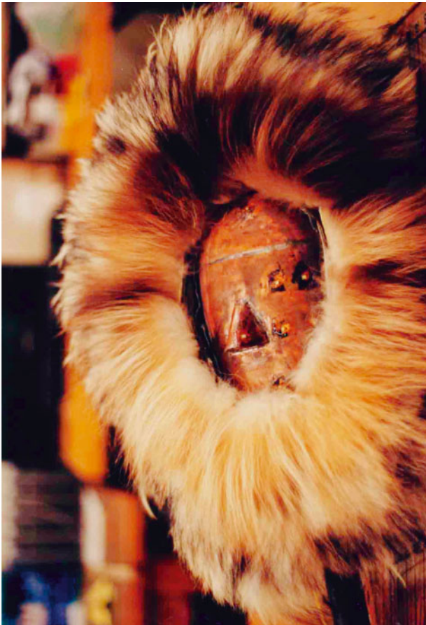
Fig. 6. Copper model with fur ruff. The ruff is positioned with respect to the copper cylinder. The thermocouples are also visible on the right side of the photograph, between the nose and the fur ruff
