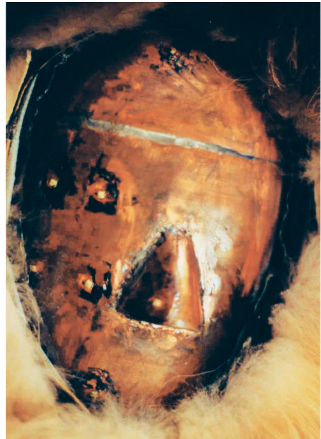
Fig. 5. Copper model with thermocouples. The white areas (Teflon) represent the location of the thermocouples used to take the heat-transfer measurements
