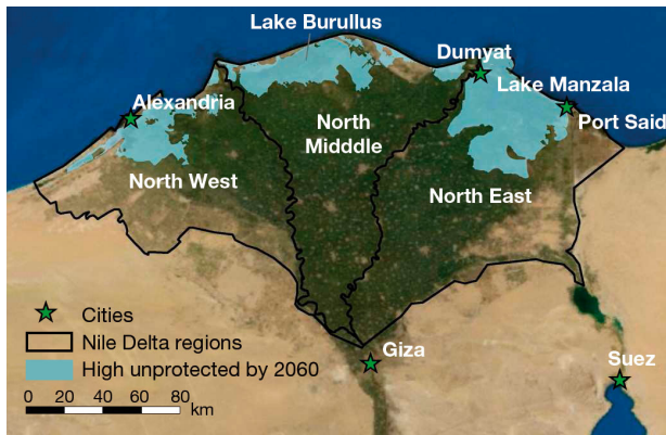
Fig. 2. Area in the Nile Delta at risk of inundation from high sea level rise (SLR) in 2060. High unprotected: high SLR scenario and no protection
