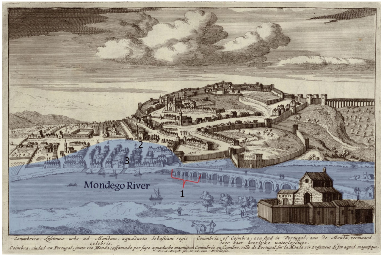
Fig. 5. Flood in Mondego valley, Coimbra, 24 February 1788 (reconstruction based on HS5, HS13 and HS37). The blue area shows the probable limits of the flood. The Mondego River covered the Coimbra Bridge, destroying 3 arches (1), flooding the downtown area of the city, where the waters reached the Santa Cruz Church (2) and damaging several buildings (3). This reconstruction is overlaid on an engraving of Pieter van den Berg, titled Conimbrica, Lusitaniae urbs ad Mundam, aquaeductu Sebastiani regis celeberrima , ca. 1720 (available at http://cartotecadigital.icc.cat/ ), based on Georg Hoefnagel's drawing (1566/67) published by Braun in Civitates Orbis Terrarum (Vol. 5, c.1598)
