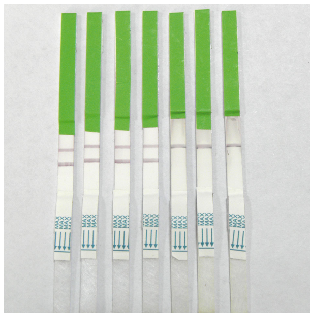
Fig. 4. Detection limit of the immunochromatographic strip. SCR standard solutions were tested at concentrations of 0, 10, 20, 40, 50, 75 and 100 \text{ } \mu\text{g ml}^{-1} (from left to right). The test line disappeared (i.e. showing a positive result) at concentrations above 50 \text{ } \mu\text{g ml}^{-1}
