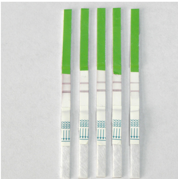
Fig. 5. Stability test of the immunochromatographic strips after storage at 4°C for (from left to right) 1 wk and 1, 2, 3 and 6 mo
