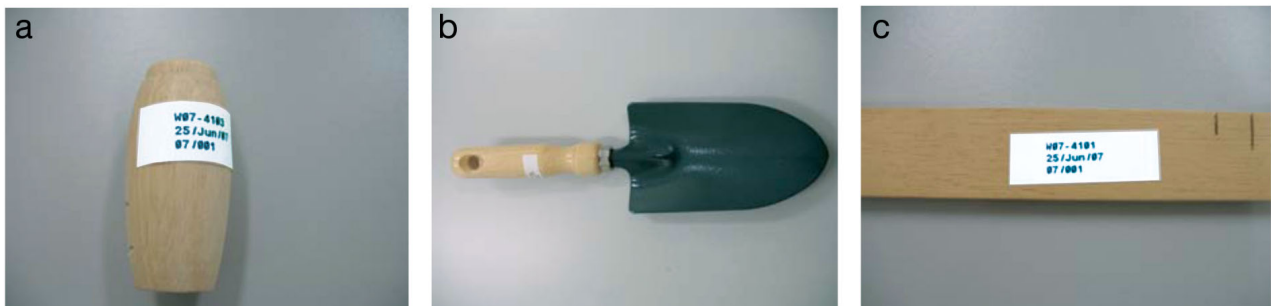
Fig. 1. Examples of previously identified processed ramin timber products: (a) window blind toggle; (b) garden trowel handle; (c) panel of window blind
