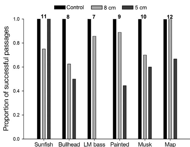
Fig. 5. Successful passage rate through 8 and 5 cm constriction rectangles as a proportion of those individuals which successfully passed through a control in the form of an unconstricted throat. The numbers above the histogram represent the sample size of individuals that passed their respective controls. LM bass: largemouth bass
