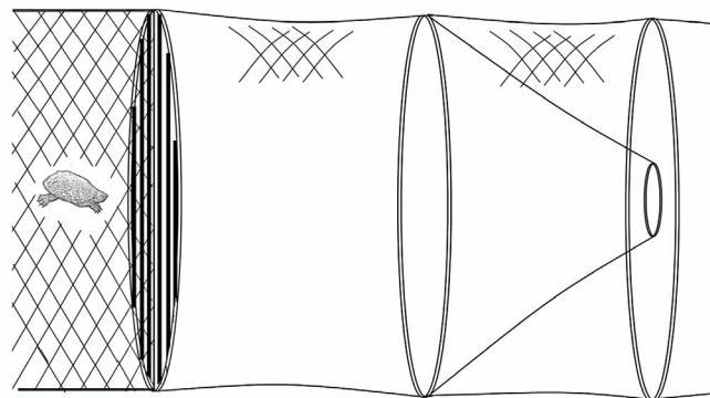
Fig. 3. Constriction rectangle (left) and vertically orientated bars (right) used as exclusion bycatch reduction devices (BRDs) for freshwater turtles in Lake Opinicon, Ontario, Canada. The height of the rectangle is 22.5 cm and the spacing of both BRDs was 5 or 8 cm
