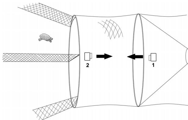
Fig. 1. Mouth of a fyke/hoop net as seen from above showing camera placement for observing pre-capture net–turtle interactions (1) and turtles interacting with the bycatch reduction device affixed to the first throat (2).
