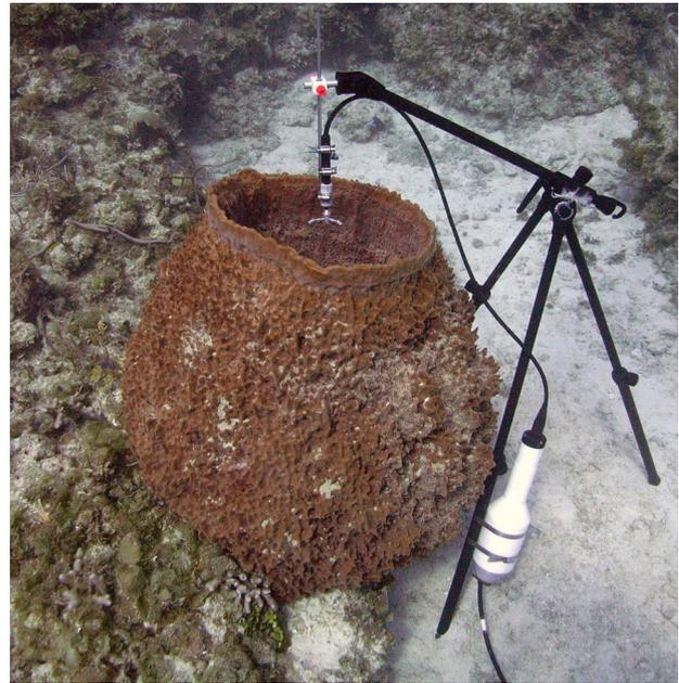
Fig. 1. The giant barrel sponge *Xestospongia muta* with an acoustic Doppler velocimeter (ADV) probe positioned over the sponge osculum to measure the velocity of excurrent seawater. Photograph: S. E. McMurray
