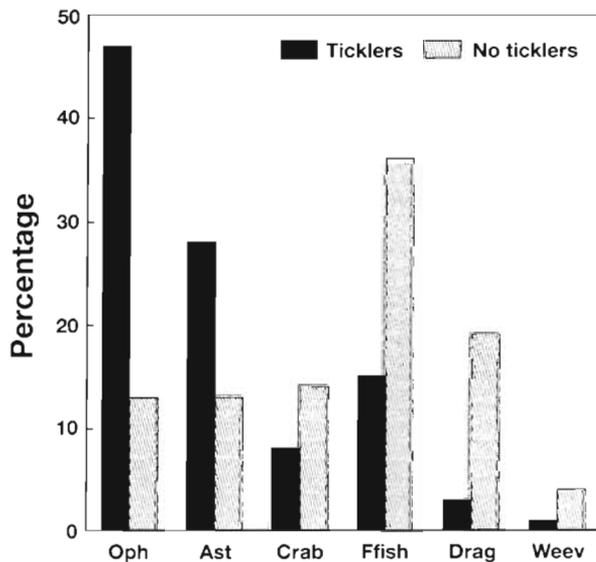
Fig. 3. Percentage of total catch accounted for by each group of animals for beam trawls fitted with and without chain mat. Oph: *Ophiura ophiura*; Ast: *Asterias rubens*; Crab: *Liocarcinus depurator*; Ffish: all flatfish species pooled; Drag: *Callionymus* spp.; Weev: *Echiichthys vipera*
