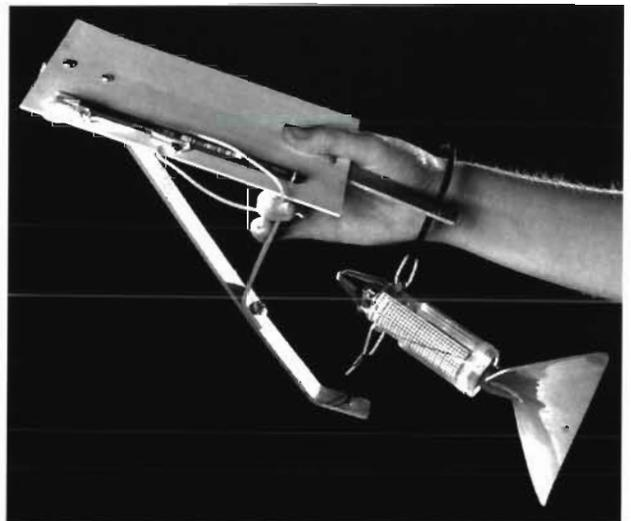
Fig. 1. Flowmeter console used to measure distance travelled. Meter was a calibrated General Oceanics Model 2030R with a low-speed rotor. Note underwater slate on top of bracket. Console was held by hand out in front of the second diver during *in situ* measurements of swimming speed
