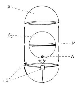
Fig. 1. The 3-D compass system. Sphere  $S_2$  was air filled while  $S_1$  was filled with silicon oil and sealed before being installed in the recording logger. M = magnet, W = lead weight, HS = Hall sensors
