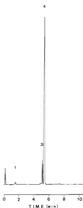
Fig. 1. HPLC fluorescence chromatogram obtained from 50 ml of a  $5.5 \text{ cells ml}^{-1}$  suspension of *Coscinodiscus wailesii* (algal diet) filtered on a  $10 \mu\text{m}$  Nuclepore filter and extracted in 2.5 ml of acetone. Injection volume =  $100 \mu\text{l}$ . Other technical details in 'Methods'. Peak identification for this and subsequent figures: (1) chl c, (2) pheophorbide a, (3) chl a allomer, (4) chl a, (5) pheophytin a
