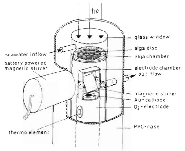
Fig. 1 Schematic diagram of the cuvette used for oxygen measurements in the field
