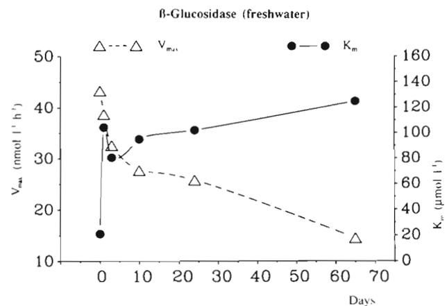
Fig. 1. Changes of  $V_{\text{max}}$  and  $K_m$  of  $\beta$ -D-glucosidase ( $\beta\text{Glc}$ ) in thawed freshwater samples from lake Große Binnensee (samples were kept frozen at  $-20^\circ\text{C}$  from 1 to 65 d)
