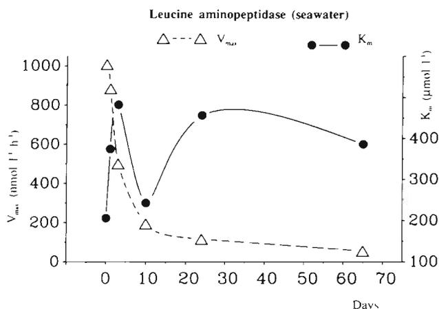
Fig. 2. Changes of  $V_{max}$  and  $K_m$  of leucine aminopeptidase (Leu-amp) in thawed seawater samples from the Baltic Sea (samples were kept frozen at  $-20^\circ\text{C}$  from 1 to 65 d)
