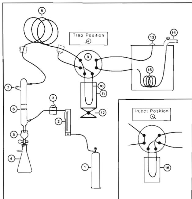
Fig. 1. Gas trapping and analysis system used in the present study. 1, Helium sparge gas; 2, rotometer; 3, toggle valve; 4, vacuum flask; 5, Omnifit 2-way valve; 6, porous glass frit; 7, crimp seal port; 8, Nafion dryer; 9, Valco 6-port valve; 10, sample loop of 1/8" (3.2 mm) Teflon tubing; 11, dewar with liquid  $\text{N}_2$ ; 12, lab jack; 13, GC injector port; 14, flame photometric detector; 15, analytical column; 16, dewar with hot ( $> 70^\circ\text{C}$ ) water
