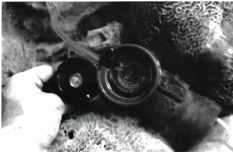
Fig. 1. Oxygen cuvette mounted on a coral reef in the surf zone. The cap with the LED is held beside the  $O_2$  cuvette. The algal disc is located in the middle of the plexiglass cuvette facing the sky
