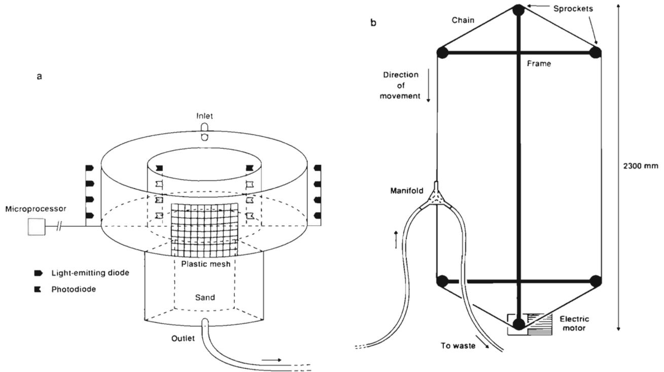
Fig. 1. Schematic diagram of (a) one prawn activity chamber, and (b) apparatus used to create the pressure cycle
