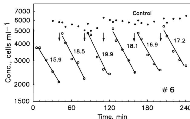
Fig. 3. *Halichondria panicea*. Reduction of algal cells due to grazing of Sponge #6 in a beaker with 900 ml seawater (12 °C) and a control beaker without sponge. Arrows indicate additions of algal suspension to the experimental beaker with sponge. The slope of regression lines represents the sponge's filtration rate ( $\text{ml min}^{-1}$ , indicated for each line)
