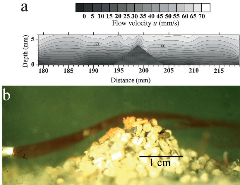
Fig. 3. (a) Horizontal flow velocity component ( $u$ ) measured with a laser Doppler anemometer close to *Heteromastus filiformis* fecal pellet mound; (b) flow patterns round fecal pellet mound visualized with dye-trail method
