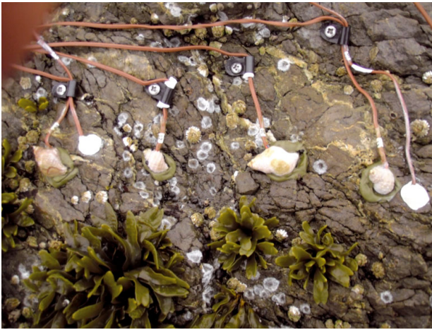
Fig. 1. Example of deployed biomimetics. The 6 biomimetic physical models deployed at the south-mid-exposed microhabitat, left to right: Nucella lamellosa , Balanus glandula , N. ostrina , N. lamellosa , N. ostrina , B. glandula . Snail biomimetics were made from empty snail shells filled with epoxy. Barnacle biomimetics consist of small dots of a different epoxy. A thermocouple sensor was inserted into each biomimetic and connected to a datalogger on land. See 'Materials and methods: Development of biomimetics' for complete details of biomimetic construction
