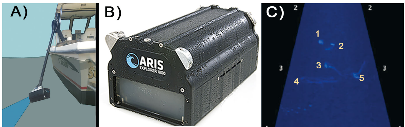
Fig. 4. (A) Sonar camera deployment using (B) the ARIS1800. (C) Example data with 5 observed Chrysaora chesapeakei jelly fish (yellow number markers)
