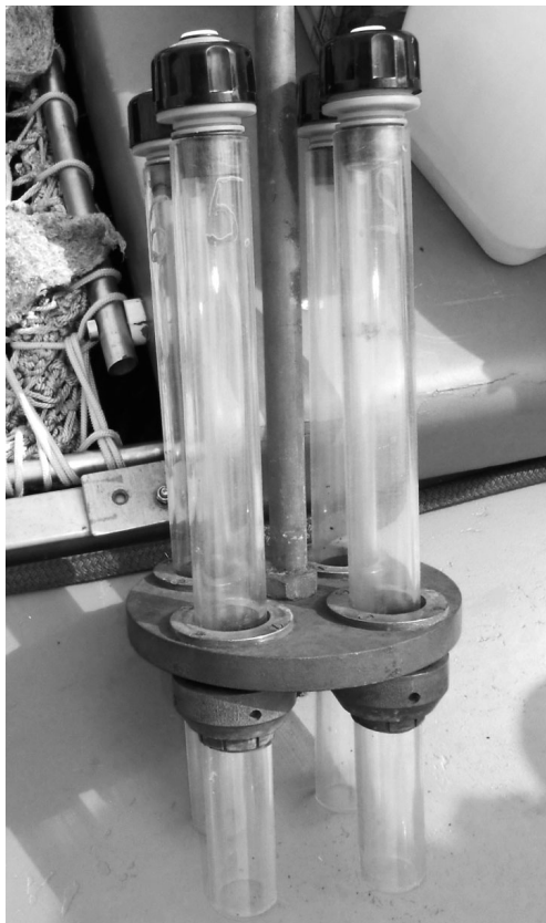
Fig. 2. Gravity corer used for collection of intact sediment–water cores
