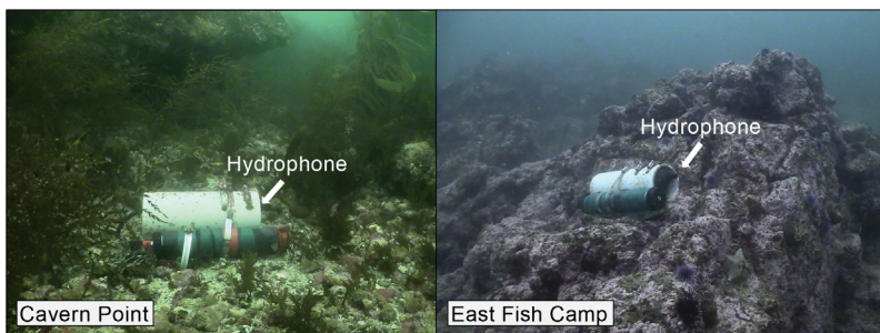
Fig. 2. SoundTrap recorder with external battery pack deployed at Cavern Point at Santa Cruz Island (protected kelp forest site) and East Fish Camp at Anacapa Island (unprotected urchin barren site). White arrows point to the hydrophone element of each recorder
