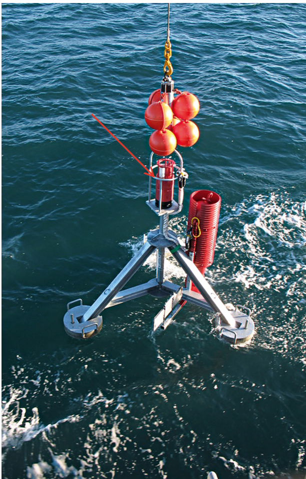
Fig. 1. One of 12 receiver deployments on large tripod landers off the coast of Plymouth, UK. The data-logging acoustic receiver is arrowed. Photo: Marine Biological Association, Plymouth
