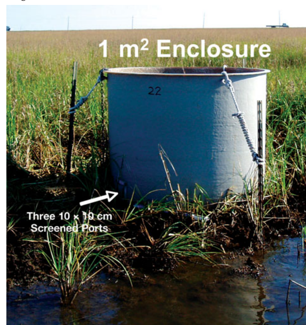
Fig. 1. Mesocosm used for growth experiments. These 1.14 m diameter fiberglass cylinders were either 1.5 or 1.8 m tall and enclosed 1 m 2 of habitat. Three 10 × 10 cm ports covered with 2 mm mesh screen allowed water exchange between the mesocosm and outside environment
