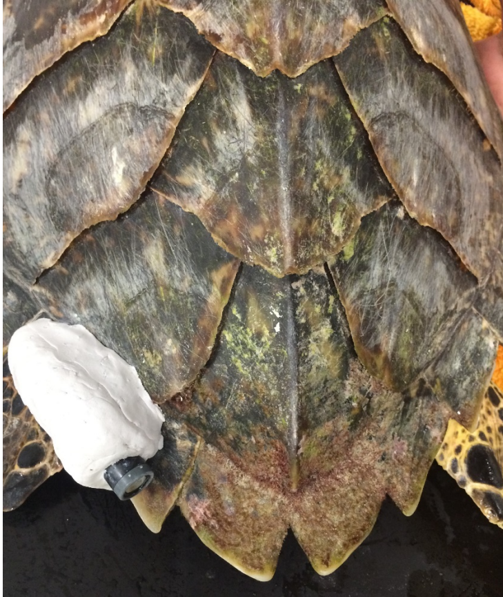
Figure S1: Attachment method for acoustic transmitters. Transmitter was attached to two marginal scutes using plastic coated wire and marine putty (white material).
