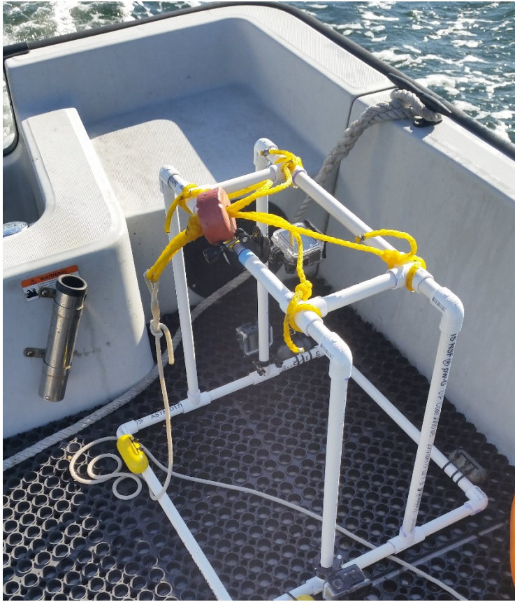
Figure S1. Video and photo system used to record oyster habitat images. The base of the frame was a 0.5 x 0.5 m quadrat and the frame was 0.5 m tall. Two GoPro™ Hero 5 cameras were mounted with a horizontal orientation and set to record video of the reef. A third camera was mounted at the top facing down and set to take still images (photoquadrats) at 30 sec intervals at the highest resolution. The quadrat was filled with sand to add weight and holes were drilled in the vertical pieces to allow water to enter/exit. Dive weights were attached to each corner for added weight.
