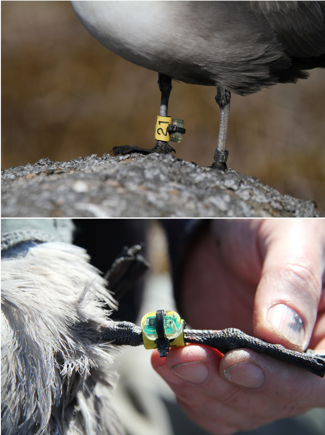
Fig. S1. Attachment of a geolocator (Intigeo-C65, Migrate Technology) on a plastic band on a long-tailed jaeger. © Yannick Seyer
